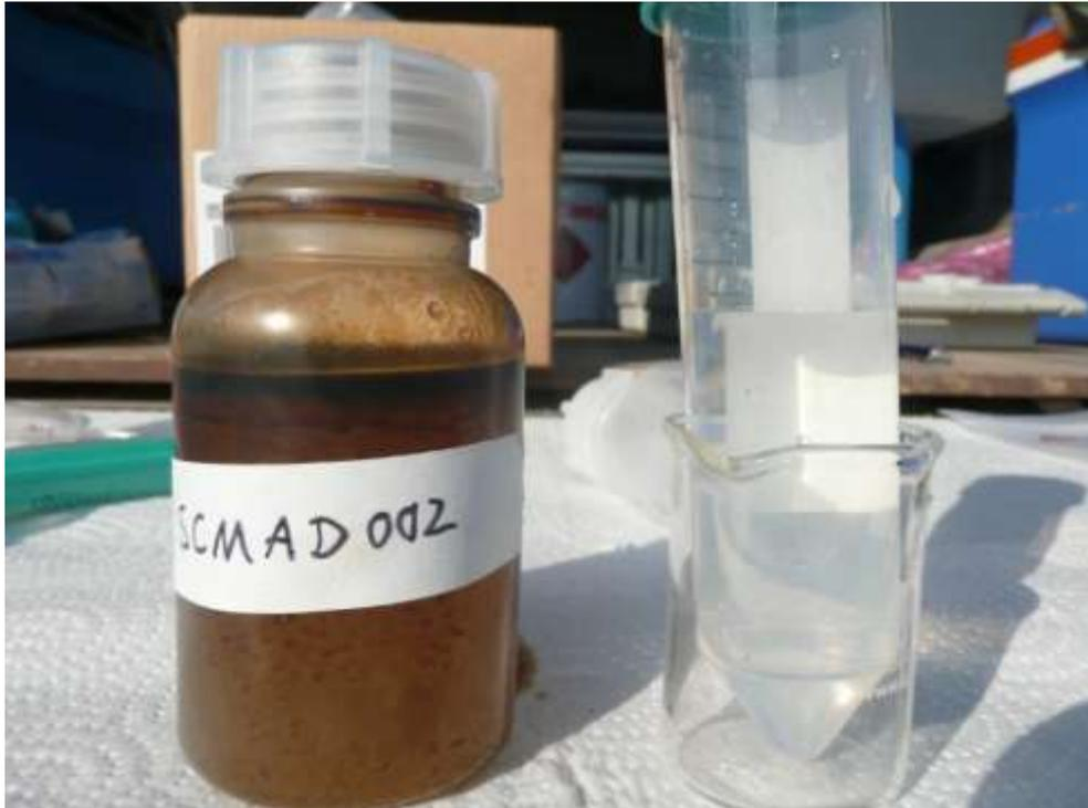
The sample in the plastic bottle left is not filtered, it has a thin floating oilphase and the brown aqueous phase below is an emulsion.
